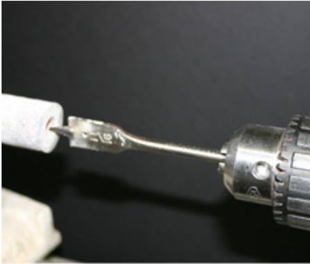
not to hit the four jaw chuck at the far end. The holes for the screw on caps are made with a 13/16 in. forstner bit (\$10). Before you drill the hole, clean up the end and make sure it is square to the lathe. Now drill a hole about 1/2 inch deep. Re-
