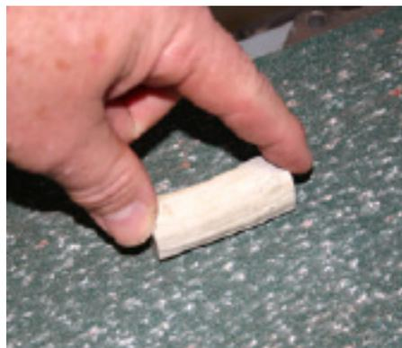
off. I very carefully hold the piece on the end with my thumb and first finger and place on a belt sander. Belt sanders can remove skin very quickly. I will form as many flat surfaces as I can on up to four sides. This should help the piece
