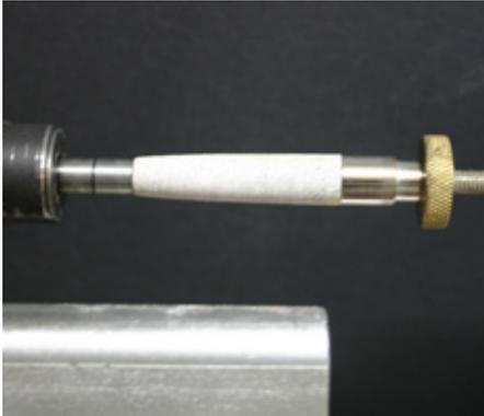
smooth taper in between. I now remove the antler from the mandrel before I sand and finish it. I do not want to sand down the bushings and get finish on the mandrel.
