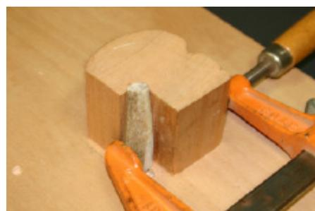
slowly and remove the bit often to clear the antler that tends to clog the drill bit. After completing the drilling, remove the piece and carefully check to see that the drill bit did not blow out the side or bottom. You are now ready to glue the tube.
