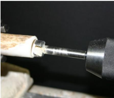
move the piece and mark it for final length. Reverse the piece in the four jaw chuck with the drilled end toward the jaw. Center with the live center and tighten the chuck. Turn the end to final length and square up the end. Drill a 1/2 inch deep hole with the 13/16 forstner bit.
