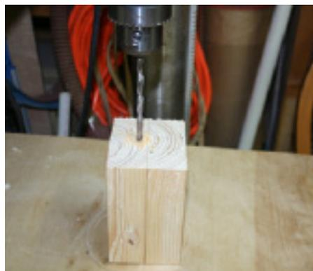
press and drill a hole deep enough so that when you pound the punch in the block, what is sticking out is shorter than the brass tube. If the rod is loose, you may have to add glue. I have reduced aluminum and iron rods down to fit the brass tube but the transfer punches are
