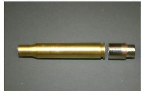
bushing for some other project that is the correct size. I have also made bushing by take an aluminum or cold rolled steel bar and drilled a hole to fit the mandrel shaft. I then turned the metal down to final size using high speed wood turning tools. High speed steel is what a machinist would use to turn aluminum or soft cold roll steel. The
