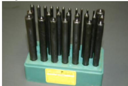
at Harbor Freight for about \$15. Find a punch that just fits snugly inside the pen tube. Find a drill bit slightly smaller than the punch or the same size as the punch. Turn the 4x4 block up on end on a drill
