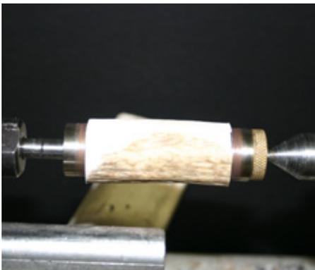
off the ends. Be sure to remove and marks left by the four jaw chuck.
