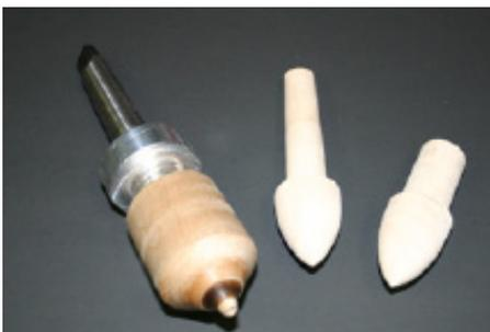
aluminum piece that has a #2 taper. Another is tapered with a turned #2 taper on the other side, and a third has a taper and shaft that fits in spigot jaws of my chuck. In the tail stock I have a tapered live center. An inexpensive center would be a good choice. Place the antler piece between centers and sand quickly with 100, 150, and 220 grit. If you feel roughness at this point or can
