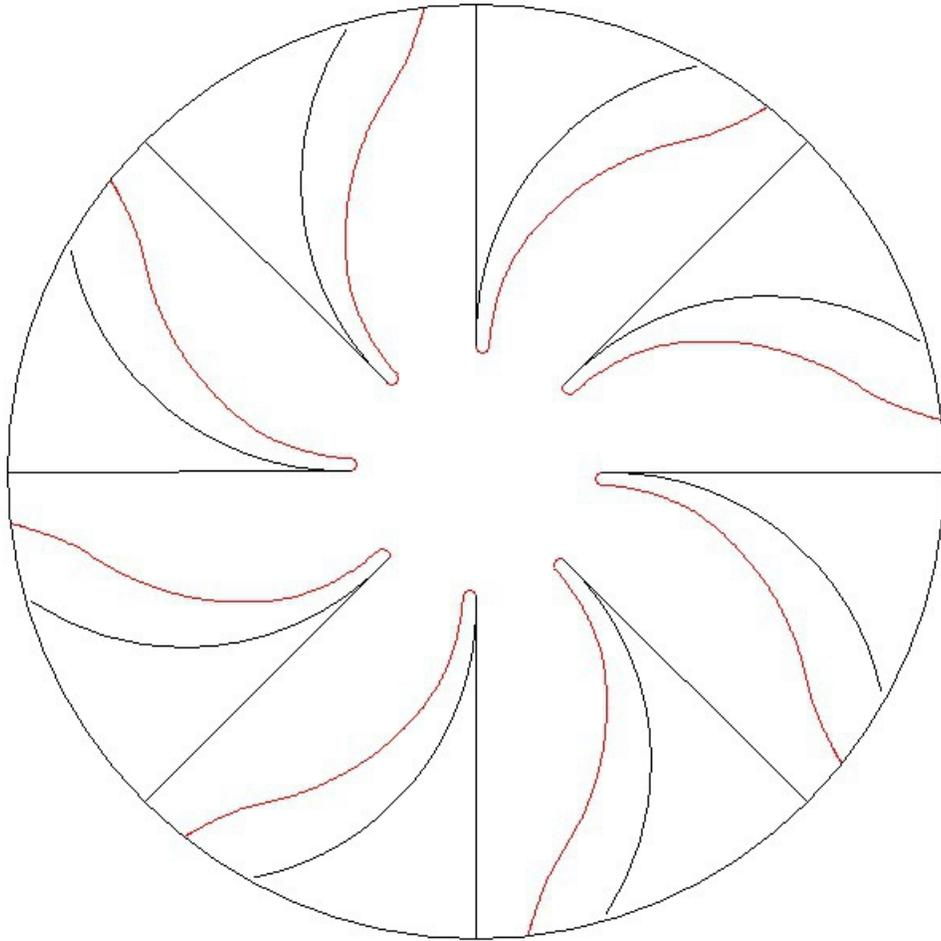
This Smith's pattern for cutting the round sanding discs. Make is smaller or larger depending upon the size of your ball by using the reduce or enlarge functions on your printer.
