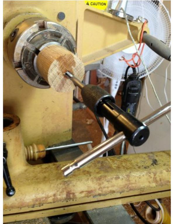
For preparing the round sanding devices, I used some salvaged white oak that I had previously rounded, cutting to approximately 2 inch lengths. I cut a tenon and put the oak in the chuck before drilling with #7 bit and tapping for  $\frac{1}{4}$  20 . With the  $\frac{1}{4}$  rod mounted in all a collet chuck, one may shape the white oak in any shape desired.
