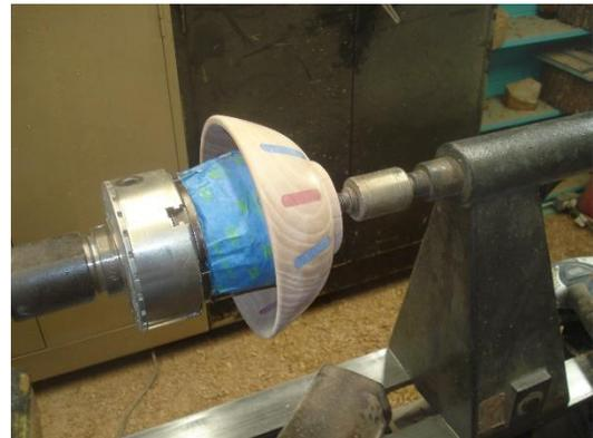
Finish – I finish with Deft Lacquer (Satin) – Apply lacquer – rub with steel wool – spray lacquer– rub with steel wool – etc – I will continue this process until I am satisfied with the finish and the look of the piece.
