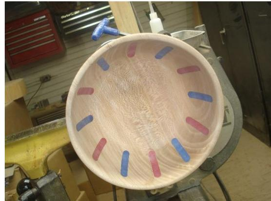
Sand piece to finish – Jam chuck – check outside of bowl and finish the base.
