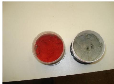
Take equal amounts of Part A and Part B and mix them together – Have a small dish of water handy to make the process smoother – after mixing – Place the Apoxie Sculpt in the flute and be sure and push it to the bottom of the flute – Need some overlap of the Apoxie Sculpt – After filling all the flutes, it will require at least 24 hours to completely set and harden.
